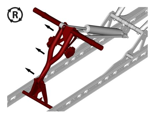
Remove and keep both (2) tubes and the long screw.
