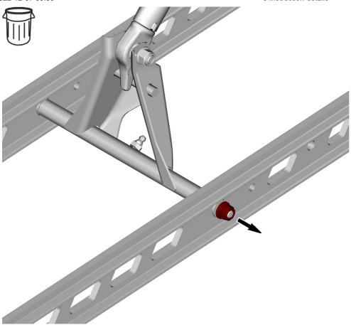
Remove original tMotion arm. Keep for reuse.
